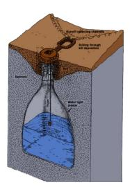
stone. With no light or air, the bacteria would die, and the sediment would settle to the ground, leaving purified drinking water in the cistern.
